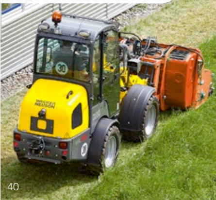
Effective green maintenance: flail mower with collection tray.
