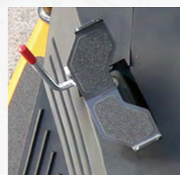
1st aux. piping pedal
